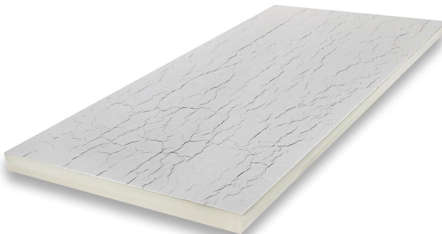
PIR is manufactured as a result of liquid ingredient foaming reaction (mainly organic ingredients from polyol and isocyanate groups) with an addition of an active foaming agent. This compound is continuously fed between two linings that limit the foamed volume.
