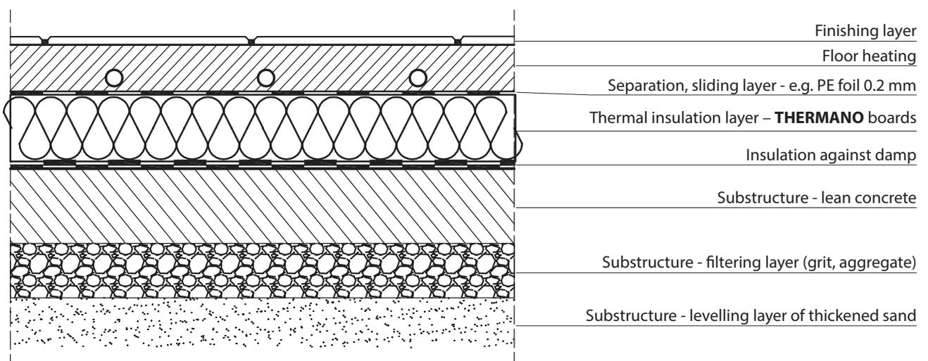
While making floor heating on **THERMANO FLOOR** take special care and seal board joints and expansion joints at walls and around posts with aluminium tape.
