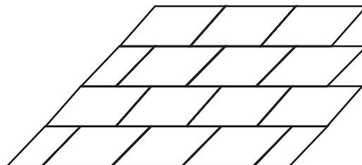
Lay the boards very carefully avoiding gaps in the thermal insulation layer. Any possible glitches may be filled with low pressure polyurethane foam.
