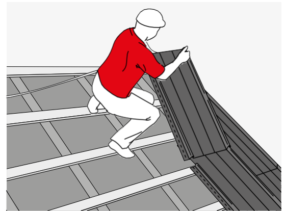
FIG. 27. LAYING THE NEXT PANEL OVERLAPPED
