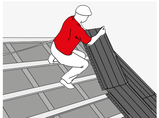
FIG. 23. OVERLAP FOR LENGTHWISE PANEL JOINTS
